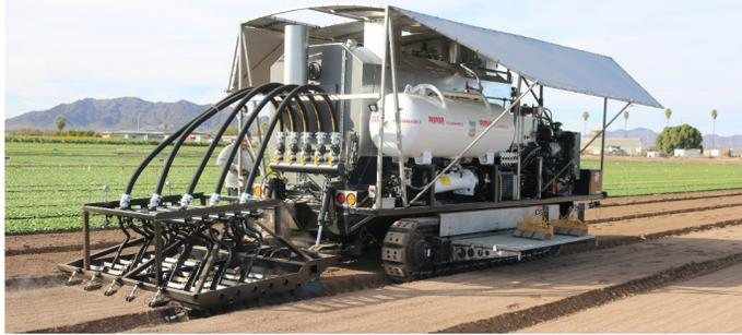
Figure 1. Tractor towed steam applicator tested in 2022 and 2023 (top). Self-propelled commercial scale steam applicator in Yuma, AZ Feb. 16, 2024 (bottom).
