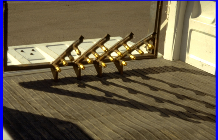
SPRAY NOZZLES FOR MULTIPLE DEPTHS OF INJECTION
